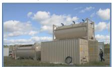
for mobile deployment. Our robust technology removes total suspended solids (TSS) such as oils, grease, metals, BOD, COD and VOC. Following primary treatment, flow water can be recycled, deep well injected or channeled for advanced treatment. It is ideal for pretreating drilling fluids and flowback to remove TSS for additional fracking, Likewise, AquaTex<sup>TM</sup> COG can pretreat produced
